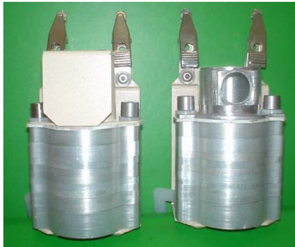
**Figure 4** Original Marple cascade impactor (left) and modified-Marple cascade impactor with equivalent to the IOM head
