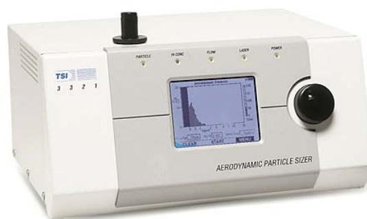
**Figure 2** Photograph of the APS Model 3321 (TSI)
