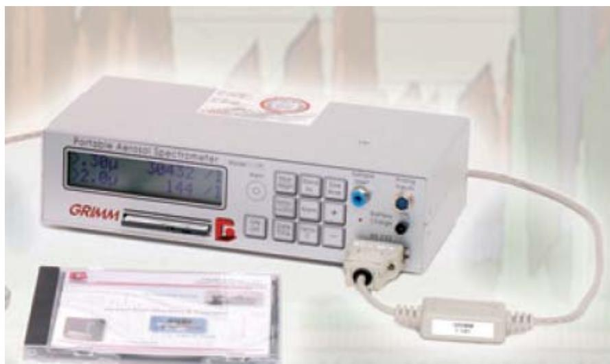
**Figure 1** Photograph of the Grimm aerosol spectrometer Mode 1.108 (courtesy of Grimm Aerosol Technology, <http://www.grimm-aerosol.com>)
